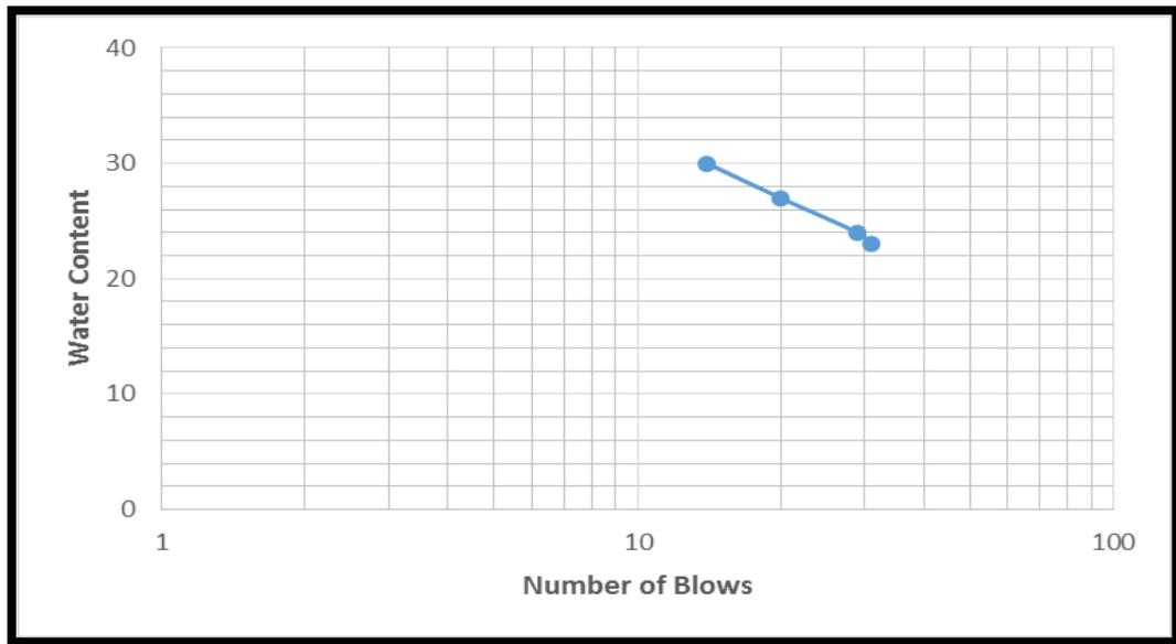
Fig2. Liquid limit test
