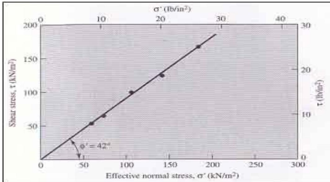
Fig3. Direct shear test
